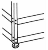
(2) To install four angle irons on four edges of bottom plate separately, then assembling the central plate, please noted the smaller bolts should be used.
